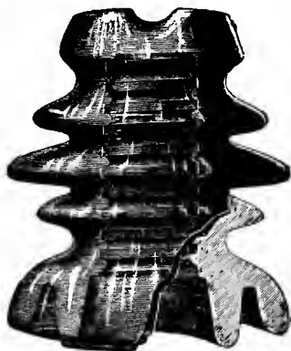
FIG. 249.—C. S. Double Transposition Insulator.
